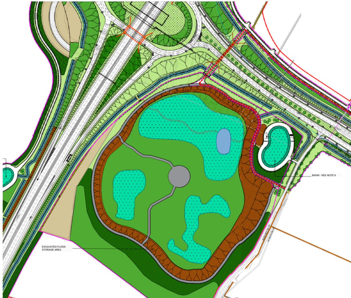
Figure 2-16 200,000m 3 reservoir in Scheme design
